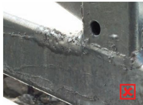
Zinc runs. A poorly placed vent hole has allowed a zinc build up inside the tube which has run out and solidified when the frame has been drawn out of the bath. **Tip: when in doubt, please ask!**
