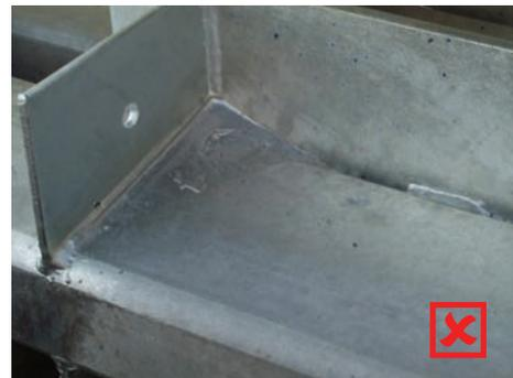
Zinc pooling. Expensive, unsightly and may interfere with erection on site. **Tip: Once again, a simple cut-out in the corner of the welded plate helps.**
