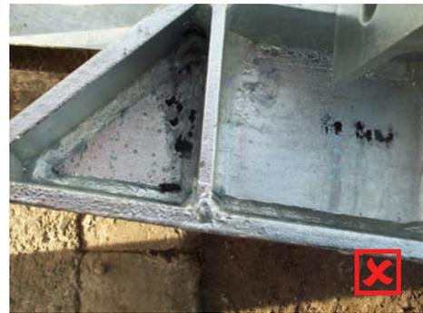
The ash and reacted flux (formed during the galvanizing process) cannot escape from this 'pocket'.
