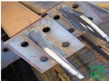
Perfect venting. Very large holes in each corner of the base plate will allow fast immersion and drainage of zinc for the perfect finish.
